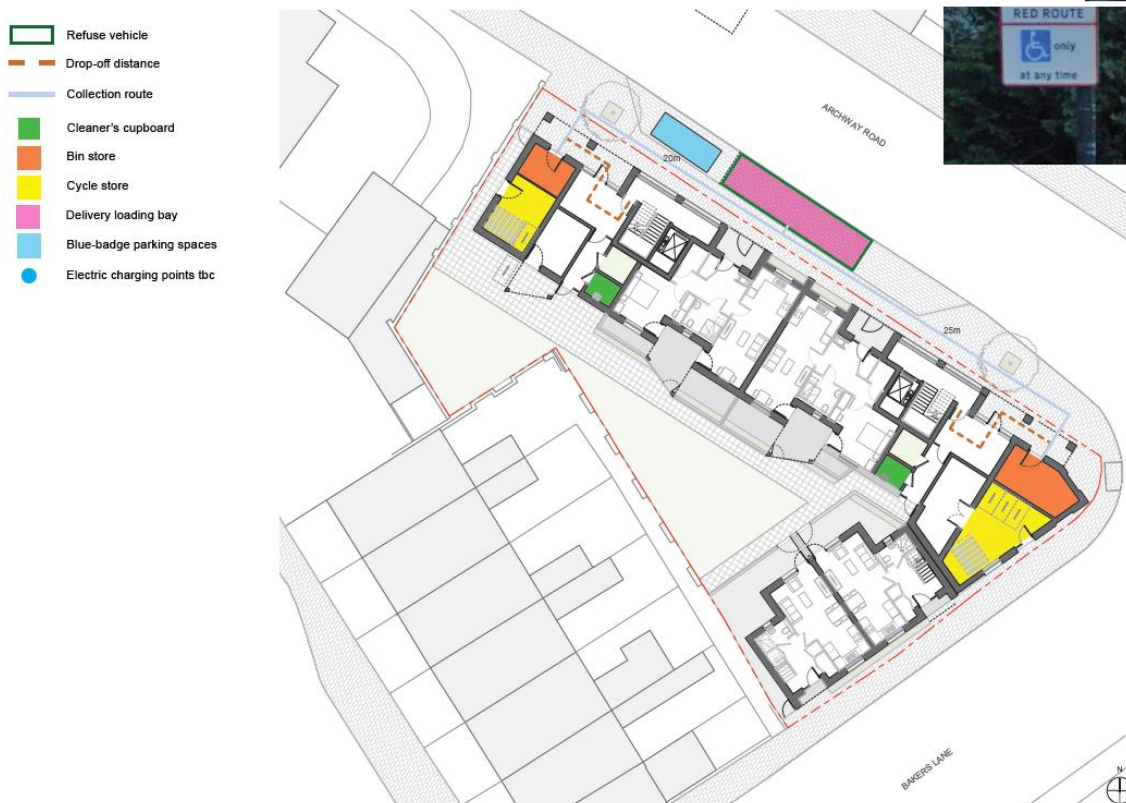
Image 5: Access, servicing, cycles and refuse
